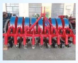
machine works on the principle of Ricewheat seeder equipment or Drum seeder, where the seed kept in rotating seed box comes out through circular holes engraved on the periphery of the seed box due to gravitational force. The rotation of seed box causes thrust on
