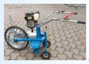
rotor rotates in direction opposite to each other's at high speed so as to generate centrifugal force. Due to the centrifugal force, the blades churn the soil and weed is uprooted completely from roots. Further the blades throw
