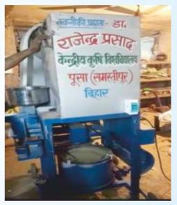
The capacity of machine is 8-10 kg/h in rice, 8-12 kg/h in wheat and 1.75-2.0 kg/h for barnyard millet. It has the ability to complete all works that are usually performed by the traditional Okhali. The machine was designed with aim to promote processing of millets in general and barnyard millet in specific. This machine is also suitable for removing skin and husk of wheat and paddy for preparation of suji, dalia and rice, respectively.
